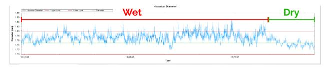
**Problem**: Oscillatory filament diameter measurements. **Cause**: Guide bearings not set properly.
