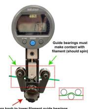
Turn knob to lower filament guide bearings
