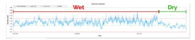
**Problem**: Oscillatory filament diameter measurements.
